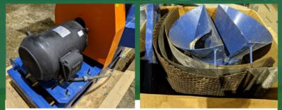
One (1) Hippo Hammer mill (Includes: steel base frame, adj. motor base plate, pulley guard cover, motor/mill pullets & drive belts, material handling fan, duct work connections & hardware, material collecting cyclone, dust bag, dust bags holder, support stand & operation manual
